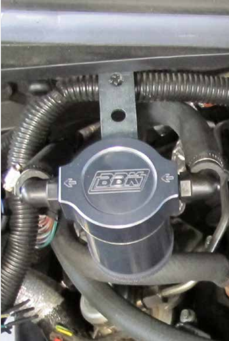
Install the BBK oil separator onto the bracket mounted to the firewall with the arrows pointing towards the passenger side fender.
