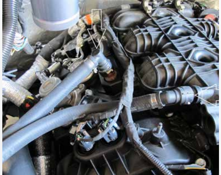
Using the hoses supplied in the kit connect the hose with the 45 degree fitting onto the intake manifold, install the hose with the 90 degree fitting onto the valve cover.
