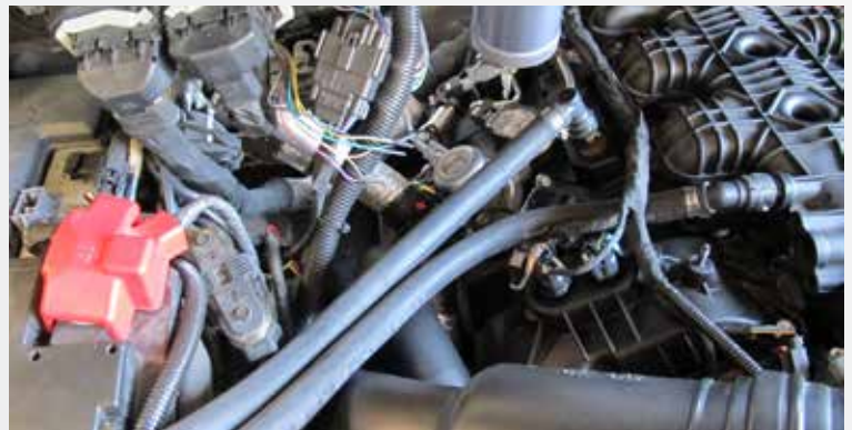
Lay the hoses parallel to each other with them going toward the negative battery terminal.
