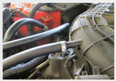
Make sure to use supplied clamps at engine connections.
