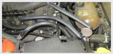
Remove factory PCV hose then install Oil Separator Kit as shown in picture. Making sure the shorter hose goes to intake manifold/draw side.
