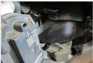
Remove factory PCV hose behind throttle body, now assemble oil separator kit as shown on front page. Make sure to hook up hose from the draw side of the oil separator to the intake manifold.
