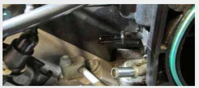
Remove factory air box and throttle body to help in removal of factory crossover hose and install of BBK oil separator kit. Remove factory hose by pushing aside the factory clip and pull outwards.
