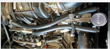
Assemble Oil Separator Kit as shown in pic making sure hose that runs to the intake manifold is the draw side shown in pic. Then remove factory engine cover and factory PCV hose. Now mount Oil Separator Kit using existing engine stud and hoses with supplied nut and clamps as shown in pic.
