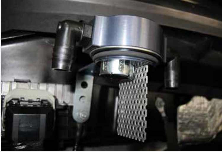
Install the BBK oil separator lid and lower catch can onto the bracket.
