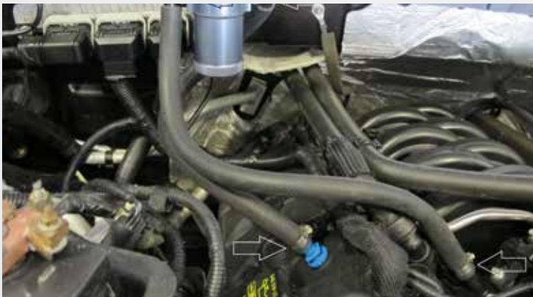
With the oil separator in place and the arrows on the lid pointing towards the passenger side fender, you can now install the vacuum hoses and clamps supplied in the kit.
