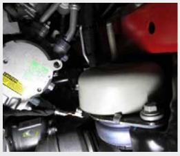
bolts that hold the actual motor mount isolator to the chassis as the entire motor mount assembly needs to be removed on the passenger side to allow room to install the BBK Header on all years from 2011 to 2015
