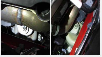
Remove the air filter box. Remove the first and second nuts on the top row of studs on the stock header of the driver side. On the passenger side, remove the first top nut that is behind the AC hose. Loosen the motor mount nut that faces up towards the header on each side, however do not remove completely at this time STEP 3
