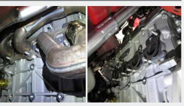
Remove the remaining exhaust manifold nuts then remove the exhaust manifold along with the gasket from the vehicle.
