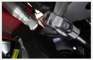
Remove the 2 bolts from the steering U-joint at the rack and pinion. Then pull the coupler downward towards the rack and pinion to separate the steering shaft from the coupler allowing the steering shaft to hang out of the way to the side.
