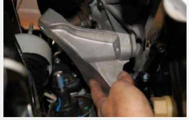
Utilizing a jacking device and a block of wood under the bell housing, remove the previously loosened nut on the driver side motor mount , once removed jack the engine upward enough to clear the motor mount stud. Remove the 4 bolts that secure the aluminum mount to the engine block and remove from the vehicle.
