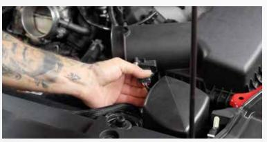
Unplug the Mass Air Sensor. Detach the Mass Air Sensor wire harness from the side of the air box by slightly pulling on the harness on the barbed mounting pin.
