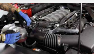
Disconnect the 3 breather hoses and the sound hose from the inlet tube. Loosen the clamps on the inlet tube at the throttle body and the air box, remove the inlet tube from the vehicle.
