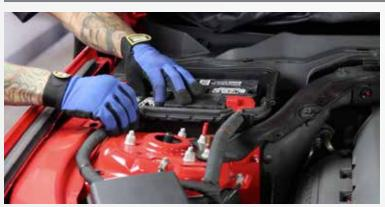
Re-install the engine cover and the radiator cover. Reconnect the negative battery terminal.
