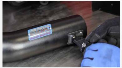
Remove the Mass air sensor from the stock air box and install it into the BBK Cold Air Tube using the supplied hardware. (The sensor will only go in one way) Install the angled BBK coupler with the vacuum port in it onto the throttle body. Install the supplied vacuum adapter onto the hose and insert it into the hole on the side of the BBK coupler.
