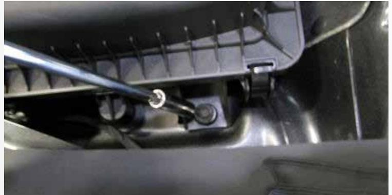
Remove the 10mm bolt on the right side of the air box that mounts it to the inner fender. Detach the air box from the lower inlet tube on the side of the radiator as you remove the air box. By pulling upwards and towards the firewall.
