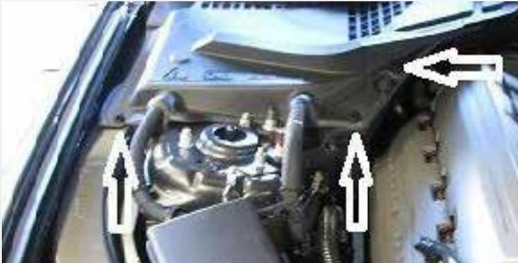
Remove the 3 screw pins that hold the battery cover to the body lift up the battery cover and disconnect the negative battery terminal.
