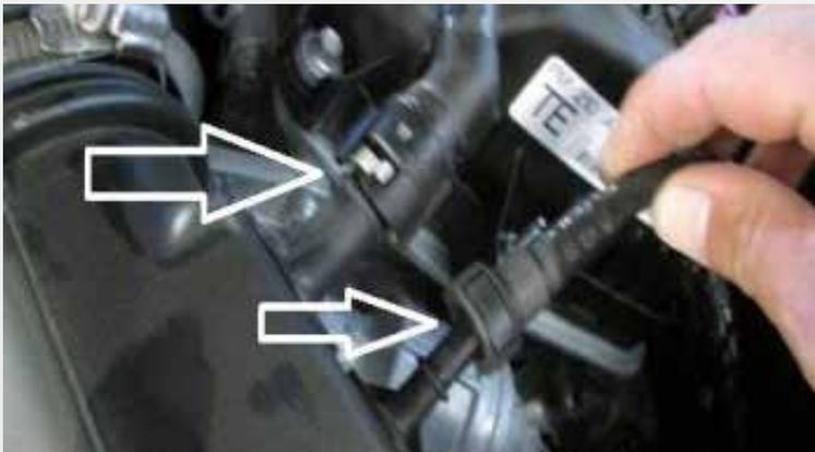
Disconnect the 2 breather hoses from the inlet tube. Loosen the clamps on the inlet tube at the throttle body and the air box, remove the inlet tube from the vehicle.
