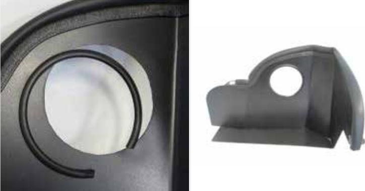
Install the supplied small trim into the hole that the BBK cold air tube will run through cut off any access. Install the supplied spongy trim to the top of the Air Filter Shield and cut off any excess trim.
