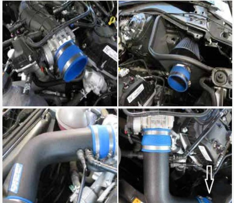
Install the tapered BBK coupler onto the throttle body and the supplied clamps. Install the BBK Air Filter thru the hole in the air shield. Install the BBK coupler and supplied clamps. Be sure that the coupler and clamps are on the engine side of the air shield when installing onto the air filter. Install the inlet tube into the coupler on the throttle body. Next slide the air filter onto the inlet tube and connect the (2) vacuum hose to the BBK inlet tube.
