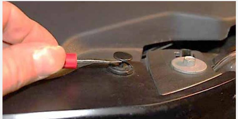
Remove the plastic radiator cover by prying up the center of the plastic pin heads at the slots cut on each side pull all the pins out and set the cover to the side.
