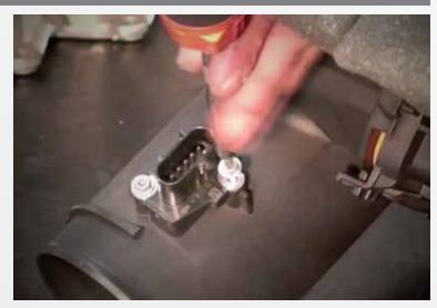
Remove mass air sensor from the stock inlet tube and install it into the aluminum mounting Block, on the BBK inlet tube with supplied screws.
