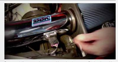
Reconnect the mass air sensor wiring plug to sensor. Route plug wiring around the back of the power steering reservoir to hide excess wire length.
