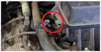
Loosen the two 10mm mounting bolts that secure the factory intake system to the vehicle. Also remove the clip on the passenger side of the stock intake system using pliers.
