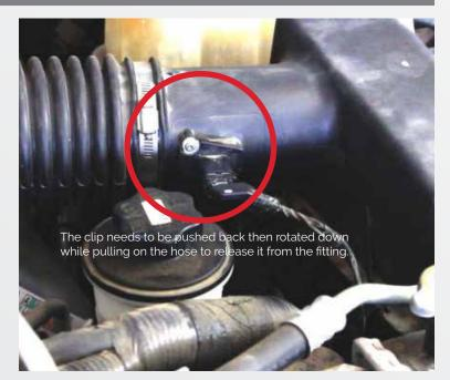
Disconnect the Mass Air Flow (MAF) Sensor.
