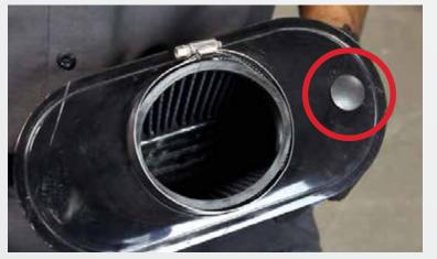
Install the sponge trimming onto the BBK Cold Air Intake shield and install the supplied plug into the BBK Air Filter.
