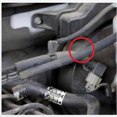
Remove the factory vent hose and replace it with the supplied 3/8" hose. Connect the supplied 3/8" hose to the plastic straight fitting on the BBK Intake Tube. The Valve Cover vent hose with the clip will be connected to the larger welded tube coming off the BBK Intake Tube.
