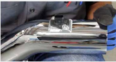
Remove the MAF Sensor from the stock intake system using a T-20 Torx and install it into the BBK Cold Air Tube using the supplied hardware.
