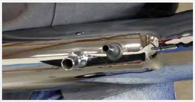
Install the supplied rubber grommet and straight fitting into the BBK Cold Air Tube.
