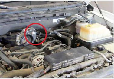
Unclip the three clips at the air box and remove the entire system out of the vehicle.
