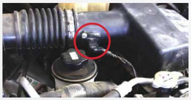
Disconnect the Mass Air Flow (MAF) Sensor.
