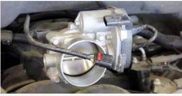
Disconnect the electrical connector at the throttle body and remove the throttle body from the vehicle.
