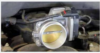
Bolt on the BBK Throttle Body and reconnect the connector.
