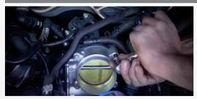
Connect the motor plug to the BBK Throttle Body and install onto the intake manifold. Use supplied bolts to secure the throttle body.
