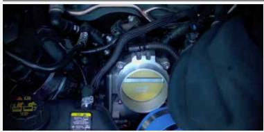
Re-install the air inlet tube and reconnect the breather tube. A little WD-40 or light grease on the inside of the tube may help in this process. Tighten the clamps.
