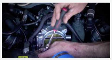
Remove the four mounting bolts from the stock throttle body, as you remove the throttle body, flip it to unplug the motor plug on the bottom.
