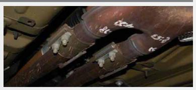
Separate the cat-back system by loosening the (2) 15mm nuts on each band clamp and prying the locking tabs up with a small flat head screwdriver while sliding the clamp towards the rear of the car.
