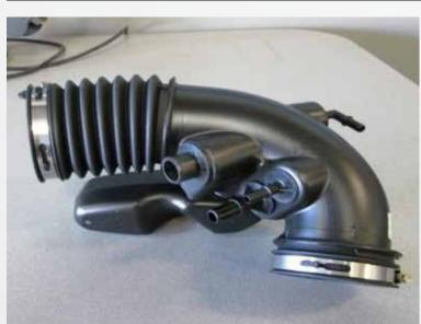
Loosen the (2) clamps on the air inlet tube at the air box and throttle body. And remove the air tube from the vehicle.
