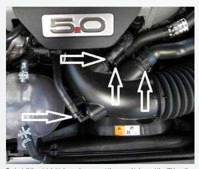
Re-install the air inlet tube and reconnect the sound tube and the (3) breather tubes. Tighten down the (2) band clamps.
