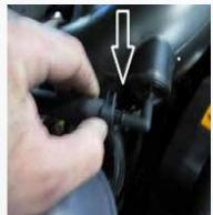
Disconnect the sound tube and the (3) smaller plastic breather hoses from the air inlet tube.
