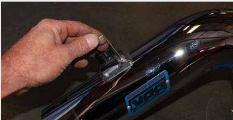
Install Mass Air sensor into the BBK inlet tube at the aluminum mount. Use the supplied Allen screws.
