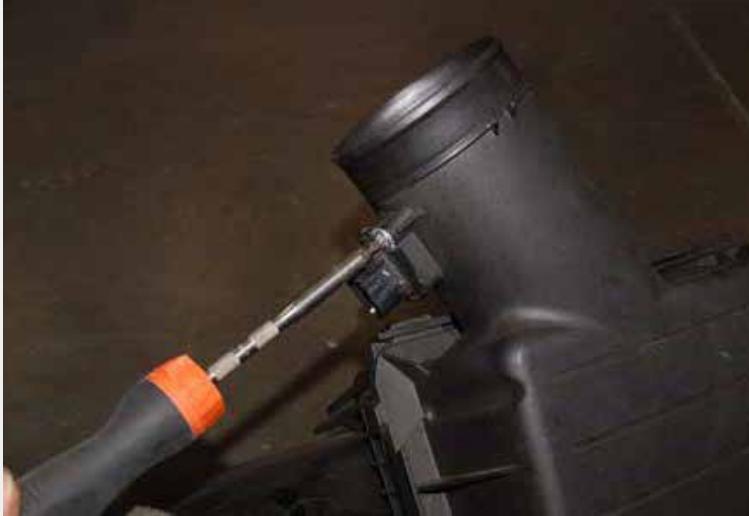
Using a Torx T20 bit, remove the Mass Air Sensor.
