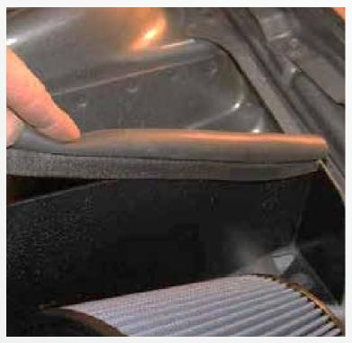
Install the supplied spongy trim to the top of the Air Filter Shield and cut off any excess trim.
