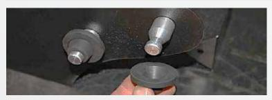
Assemble the 2 aluminum pins to the bottom of the BBK Air Filter Shield using the supplied  $\frac{1}{2}$ -20x1/2" Phillips screws. Install the stock rubber grommets onto the pins.
