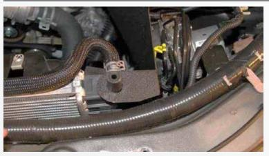
Install the BBK Air Filter Shield into place and position over the radiator mount peg with the rubber grommets seating into their holes in the inner fender. Install the stock bolt back into the small tab on the shield and tighten the bolt. Re-install the upper radiator mount and tighten the bolts.
