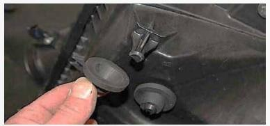
Remove the bolt on the right side of the air box that mounts it to the inner fender. Detach the air box from the lower inlet tube on the side of the radiator as you remove the air box. Detach the Mass Air Meter wire harness from the side of the air box by slightly pulling on the harness on each barbed mounting pin. Also remove the 2 bottom rubber grommet for the air box.
