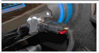
Remove the MAF sensor from the stock air box and install it into the BBK Cold Air Tube using the supplied hardware. (The sensor will only go on one way)
