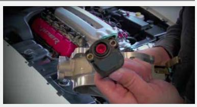
Transfer the TPS sensor from the stock throttle body to the BBK unit.
