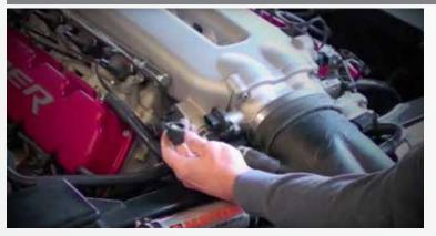
Disconnect the throttle cable from its tab by pulling forward on the black cable end.
