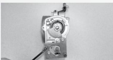
Using the puller tool remove the motor.
