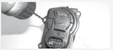
Using a drill with a 3/16 bit CAREFULLY drill out the rivets that attach the throttle body motor housing to the throttle body.
