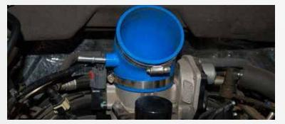
Install the blue connector and two clamps onto the throttle body.
