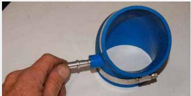
Install the provided 3/8" diameter by 2" long aluminum adapter tube. Push the long end into the port on the side of the provided blue hose connector. This is the new breather tube connection point.
