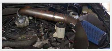
Install the chrome inlet tube into the hole in the filter shield then on to the connector on the throttle body. Rotate the inlet tube for the best position and tighten the clamps at the blue connector. Install the filter on to the end of the inlet tube and tighten the clamp.
