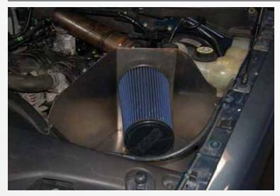
Install the BBK filter shield on the driver side inner fender. Use supplied bolts and washers to mount the shield.
