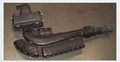
Remove the four retaining bolts for the stock air intake at the intake manifold. Remove the bolt just forward of the power steering reservoir that holds the inlet tube. Remove the assembly from the vehicle.
