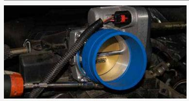
Install the supplied blue rubber hose coupler onto the throttle body. Install the clamps and Tighten the one on the throttle body.
