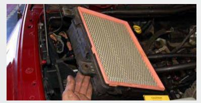
Loosen the hose clamp on the inlet hose where it connects to the decorative plenum. Release clamps on air-box lid and remove lid and inlet hose. Remove air-box bottom and Filter.
