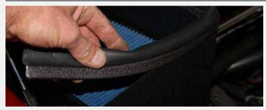
Install sponge seal to top of air filter shield. Trim off extra.
