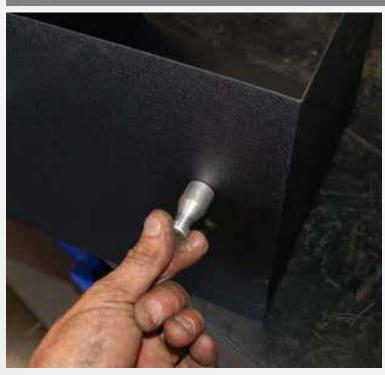
Install the supplied aluminum pins to the bottom of the air shield using the supplied screws.
