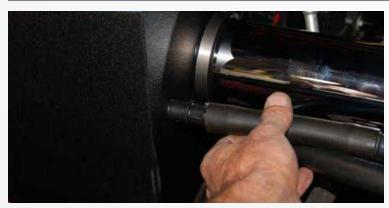
Insert the supplied 5/8" black plastic hose connector into the hole in the base of the filter, connect the stock breather hose to the black connector. If you need a little extra length In the breather hose, loosen the clamp at the other end of the hose, where it connects to the engine and turn the hose toward the air filter.
