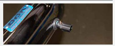
Install the supplied black rubber grommet in the chrome inlet tube. Install the Intake Air Temp (IAT) sensor that you removed from the stock plenum in STEP 2, into the grommet.
