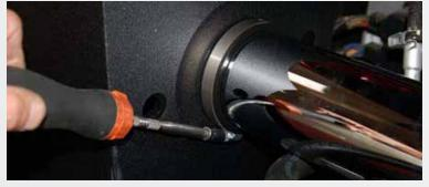
Take the clamp off the neck of the supplied air filter and place on chrome inlet tube, on the engine side of the shield. Install the filter onto the tube and line up the breather hole in the filter base with the forward hole in the shield. Place clamp on neck of filter and tighten.
