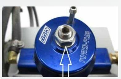
Loosen the lock-nut on the top of the fuel regulator.
