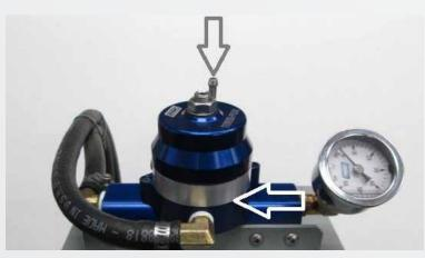
Now that the fuel system has been pressurized it is a good time to check for leaks around the BBK Fuel Regulator
