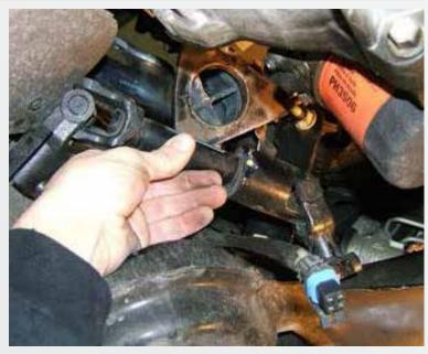
Remove the bolts that attach the steering shaft to the steering rack and firewall steering column yoke.
