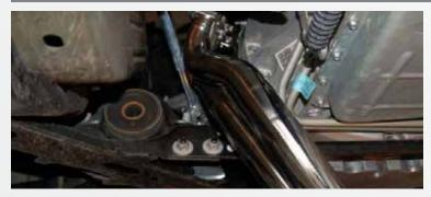
Install the BBK Full Length Headers from underneath the vehicle. They will slip right in place and onto the studs. Install all the nuts and tighten both sides.
