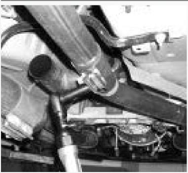
Separate the cat-back system by loosening the 2 nuts on each band clamp and prying the locking tabs up with a small screwdriver while sliding the clamp towards the rear of the car.
