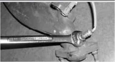
Remove the front driver side oxygen sensor from the manifold.
