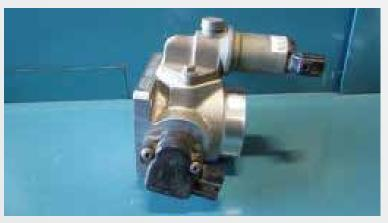
Remove the TPS from the stock throttle body. If it is equipped with an IAC valve, use the supplied gasket to swap it over to the BBK Throttle Body. Also install the TPS sensor onto the BBK Throttle Body with the stock screws.
