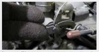
Disconnect the TPS electrical connector, the throttle cables, and the auxiliary return spring (if equipped) from the stock throttle body.
