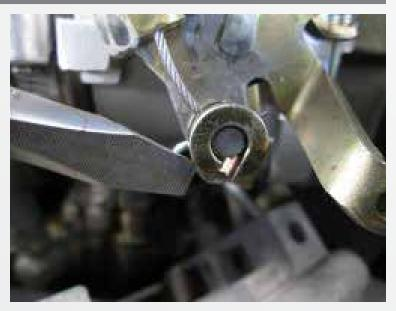
NOTE: On Ford Ranger only Install the throttle cable adapter with the open slot end facing down and install the safety clip onto the back side of the adapter.
