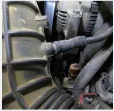
Unclamp the air filter inlet tube from the neck of the throttle body. Disconnect the breather tube and move air filter inlet tube to the side.
