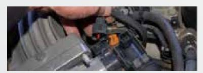
Unplug the TPS and IAC valve electrical connections.
