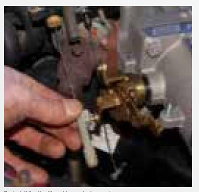
Re-install the throttle cables and return spring.
