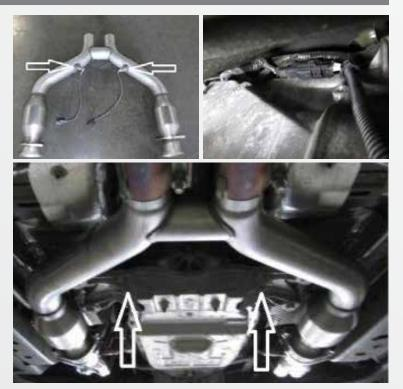
With the BBK Full Length Headers installed, remove the (2) rear oxygen sensors from the stock exhaust and transfer them over to the BBK H-PIPE.
