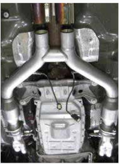
Lift the BBK H-PIPE up to the collector flanges on the headers, Connect the headers and H-Pipe utilizing the hardware supplied in the header kit.
