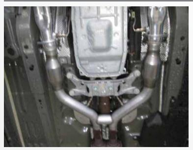
With everything in place level out the exhaust and start tightening down all the hardware and clamps starting at the collectors and working your way towards the rear of the vehicle.
