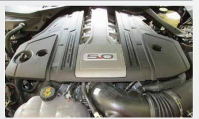
Remove the 2 black caps at the front of the Engine cover (one left side one right side) – with a 10mm socket remove the 2X 10mm nuts – then pull the engine cover up and away from the vehicle. Disconnect the 2 breather hoses and sound tube, then remove factory air tube from stock throttle body and airbox.
