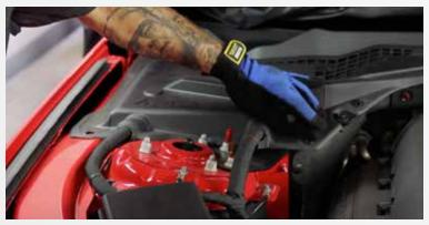
Remove the 3 screw pins that hold the battery cover to the body lift up the battery cover and disconnect the negative battery terminal.
