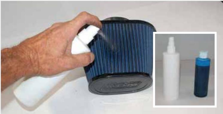
Wipe large debris from filter. Using the taller white bottle of cleaner from the kit, liberally spray the cleaner until it completely saturates the pleated material.
