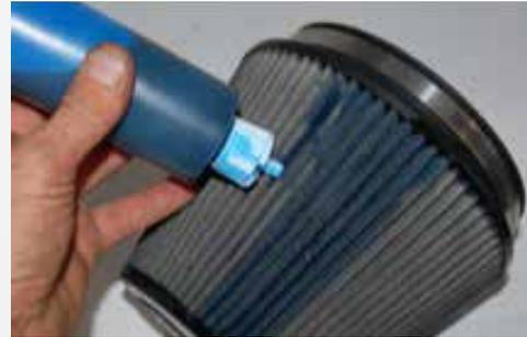
For best results, insist on BBK filter oil for your BBK filters. Using the blue filter oil from the kit, apply a bead of oil along the crown of each filter pleat. Work your way around the filter until all pleats are covered.
