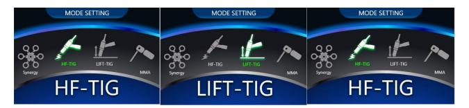
Press button or to select (or turn the red knob) the welding mode you want to do, then press to next step (or press the red knob).
