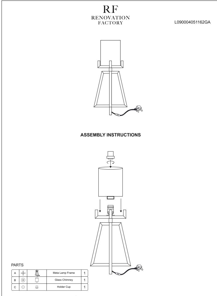
Unscrew the pre-fitted holder cup, insert glass, and re-tighten holder cup. **Warning : To avoid cracking of glass, do not over - tighten pillar cap.**
