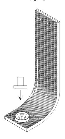
STEP 7 Assemble Glass Shade: Place the glass carefully, tighten the metal holder cap. Donot over tighten the metal holder cap.
