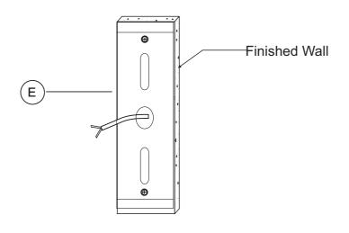
STEP 4 Connector Open : Open the connector, attach the connector to main wire. Attach the brown coloured wire to phase, blue coloured wire to neutral and green yellow coloured wire to earth.
