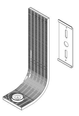
STEP 2 Installation Fixture Base: Find a desired location to hang the wall light and mark location for screws on the wall. Allign with the two holes of the wall. Place anchors on the wall on the marked points. All anchors screws must be attached directly into anchors. Tighten the screw.
