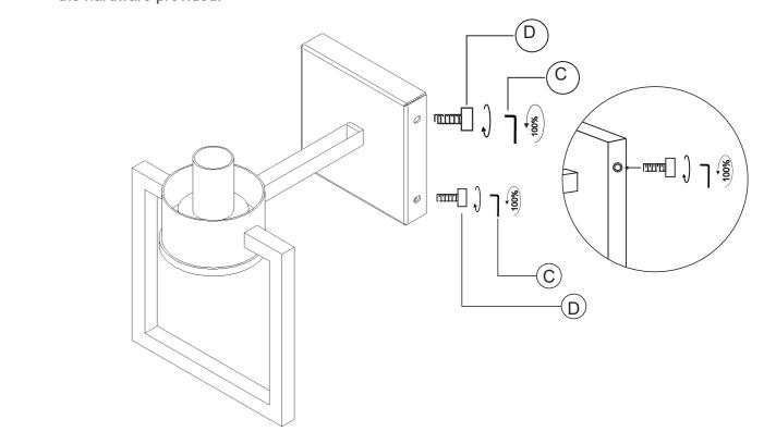
STEP 2 Installation Fixture Base: Find a desired location to hang the wall light and mark location for screws on the wall. Align with the two holes of the wall. Place anchors on the wall on the marked points. All anchors screws must be attached directly into anchors. Tighten the screw.
