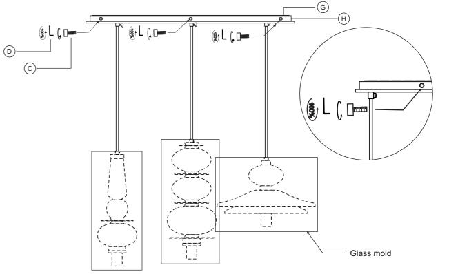
STEP 2 Installation Mounting Plate : Install the mounting plate to the ceiling using the fastener. Allign with the two holes of the ceiling. Tighten the threaded bolt.
