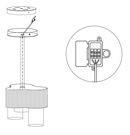
STEP 4 Attach the Main Wire: Take out the main wire through the mounting plate. Attach main wire to the connector. Attach the brown coloured wire to phase, blue coloured wire to neutral and green yellow coloured wire to earth.
