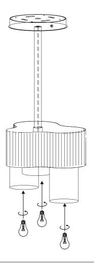
STEP 9 Restore power to junction box and test fixture.
