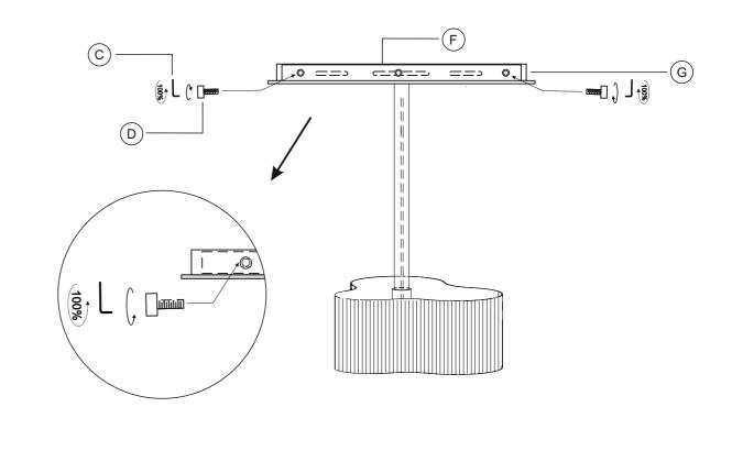
STEP 6 Unscrew Holder: Unscrew the metal holder cap gently
