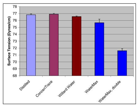
**Figure 1.** Surface Tension of Water Products. Systematic equipment error shows all surface tensions about 4 dynes/cm higher than actual value.
