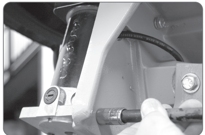
Figure 8 Shown using a 6" extension with 7/16" socket.
