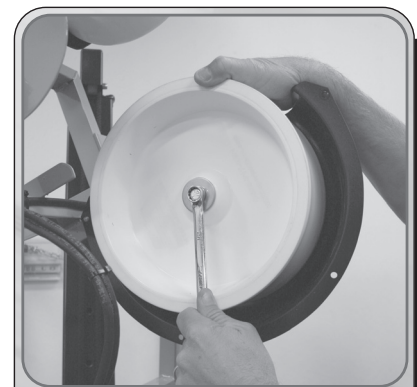
Figure 9 Hold wheel while loosening bolts.
