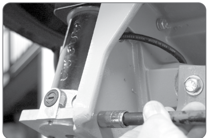
Figure 17 Shown using a 6" extension with 7/16" socket.
