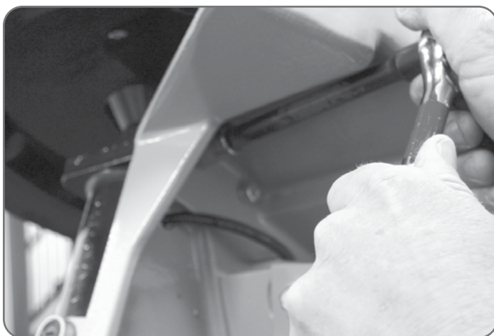
Figure 16 Shown using a 6" extension with 1/2" socket.
