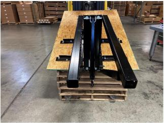
9. Bolt the H-Frame to the extension arms using (2)  $\frac{1}{2}$  x 12" hex bolts, (4) nylon washers and (2)  $\frac{1}{2}$ "
