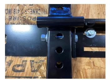
2. Next, using (2)  $\frac{1}{2}$ "x 4  $\frac{1}{2}$ " hex bolts, lockwashers, & hex nuts attach the main support channel to the front pivot tubes welded to the front of the perforated supports as shown in Figure D. **Spread**
