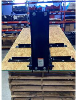
6. Attach the Lower Extension Arms using (1) ½"x 12" hex bolt, (2) nylon flatwashers and (1) ½" locknut. Place one nylon flatwasher between the extension arm and the extension arm support. The nylon washers eliminate paint wear and provide free movement at the pivot points. Remember, the nylon flatwashers go BETWEEN the extension arms and the side of the extension arm support.
