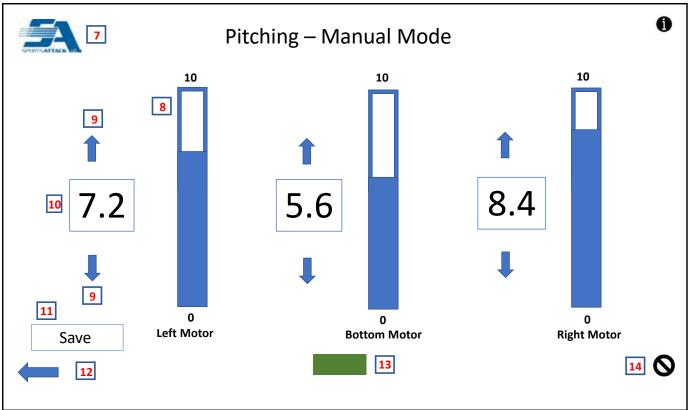
**Note**: On this screen you are able to control each motor individually. Each slider has the corresponding motor effected below it, left motor is on the left, bottom motor in the middle and right motor on the right.
