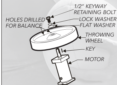
Figure 10 Hold wheel in place while loosening bolts.
