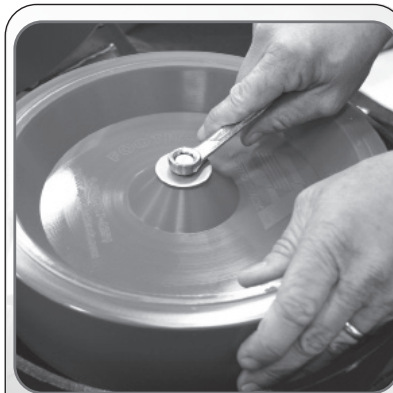
Figure 10 Hold wheel in place while loosening bolts.
