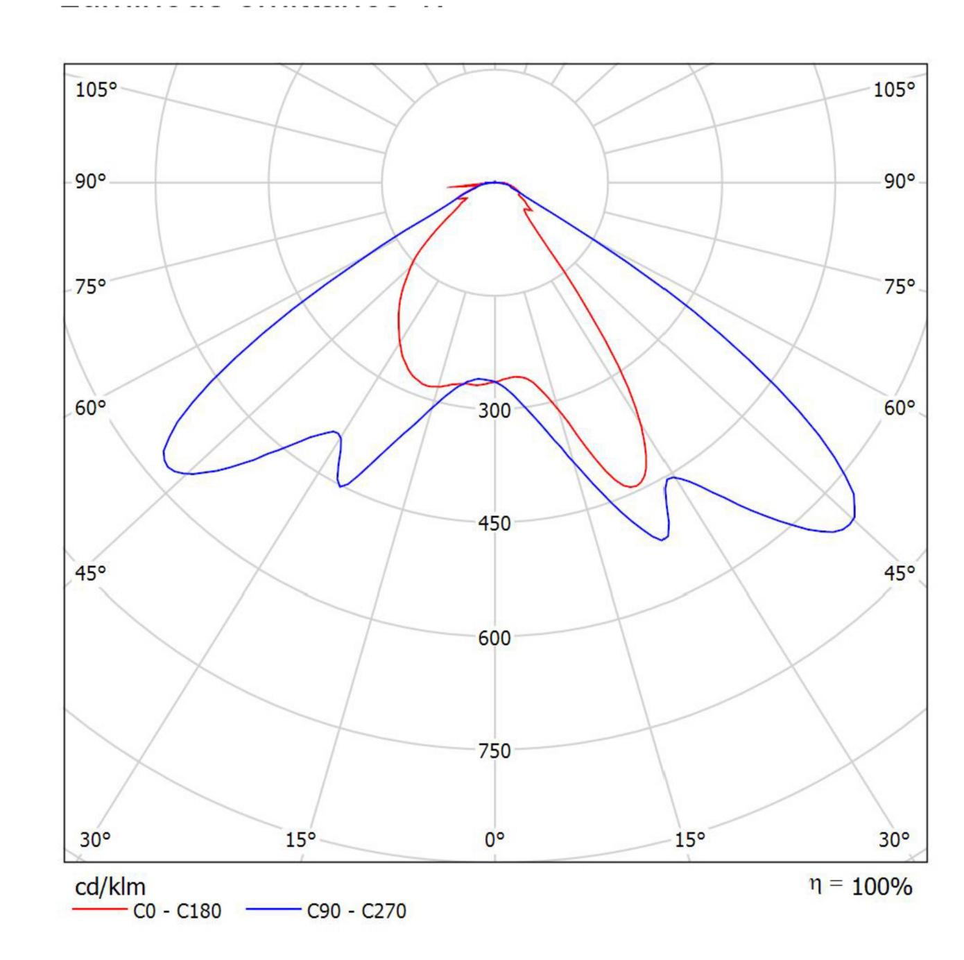
Luminaire classification according to CIE: 100 CIE flux code: 56 90 98 100 100
