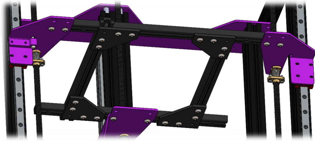
Figure 77 Underside view for the heatbed frame assembly
