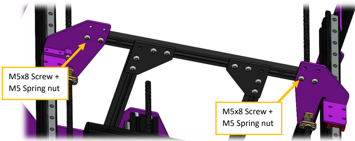
Figure 75 Underside view for the heatbed frame assembly
