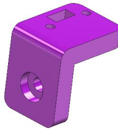
Figure 2 Y Axis endstop bracket
