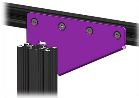
Figure 33 Final finish fixing detail, left side.
