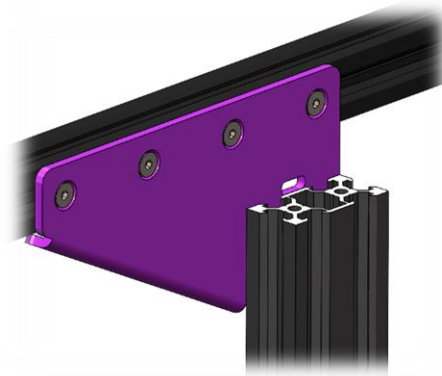
Figure 32 Final finish fixing detail, right side.
