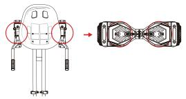
Secure your Gotrax Hoverkart to your self-balancing scooter using both adjustable straps with Velcro. With the velcro side facing away from your scooter, attach one hook of each adjustable strap to the back of each pedal mount.
