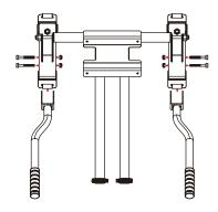
2. Insert the frame into the seat frame. Adjust the frame and the seat frame to your preferred size. Secure the frame in place using the locker.
