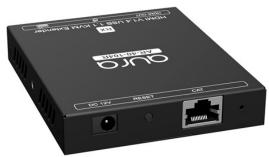
This aura HDMI USB KVM extender enables control of a workstation or PC with keyboard and mouse, whilst viewing the video source up to 120m away from the workstation or PC. It extends an HDMI signal between Transmitter and Receiver over a single CAT6 cable and supports two USB devices in the reverse direction. 4Kat 30Hz HDMI video signals up to 120m including HDCP 1.4. Supports 2x USB 1.1 signals from receiver back to transmitter for KVM functions.
