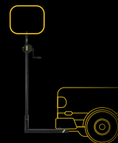
TRUCK HITCH MOUNT Includes mount and 7.5ft chain driven extension pole SD-HITCHKIT-LRG-G1
