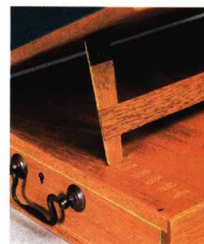
A stand that folds away. The top of the desk is mortised to accept the support stand, which is hinged to the lower writing surface.
